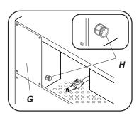
The connection needs to be made in the wiring box at the back. Remove the coverplate (G) in order to reach the connection clamps.
