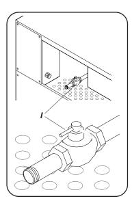
The gas supply pipe should be connected to the gas tap (I), which is on the right next to the wiring box on the back.
