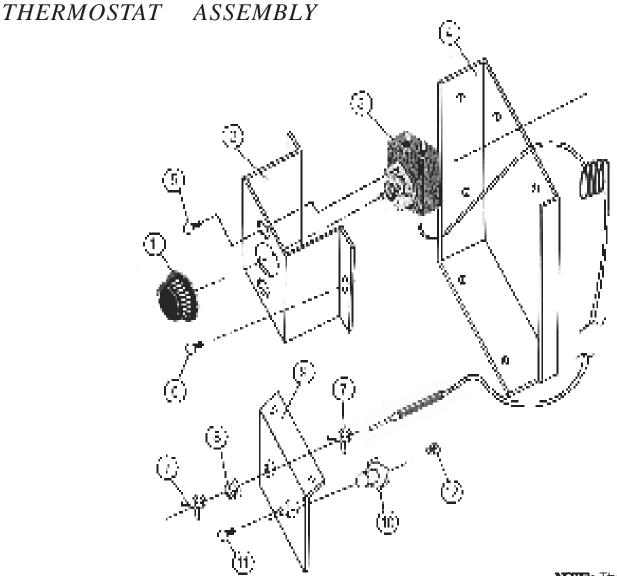
Description Ref. PartNo. No. EA-00607-0 Thermostatknob 1 2 CA-13213-0 Thermostatbracket 3 EA-00606-0 Thermostat 4 CA-13215-0 Thermostatbracketadapter 5 TU3624 Screw6-32X1/4" Screw-selfdrilling8-18X1/2" 6 TU7733 7 EA-00434-0 Clip-3/8" spring 8 EA-00608-0 Grammet/rubber 9 CA-13214-0 Plate 10 EA-00594-0 Thermostat-HI-Limit Screw8-32X1/2" 11 SB-00828-0 TU3266 Nut-brass8-32 12
