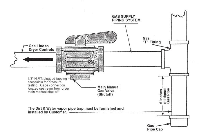
The dryer and its individual shutoff valve must be disconnected from the gas supply piping system during any pressure testing of that system at test pressures in excess of 1/2 psi (.04 bar).
