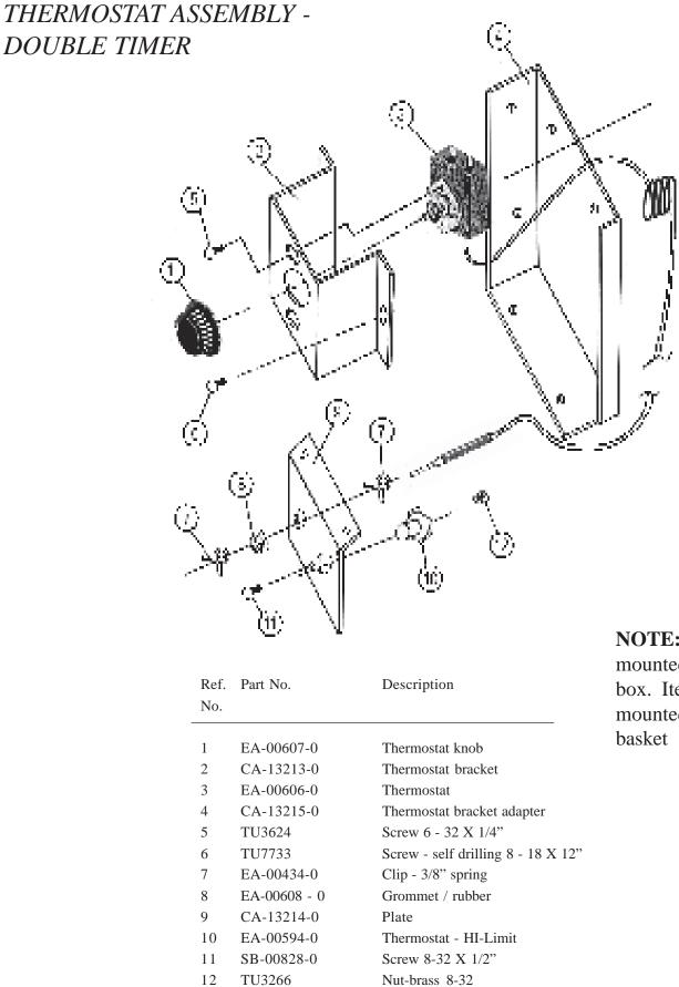
**NOTE:** Items 1 thru 6 mounted in front wire box. Items 7 thru 12 are mounted under the basket
