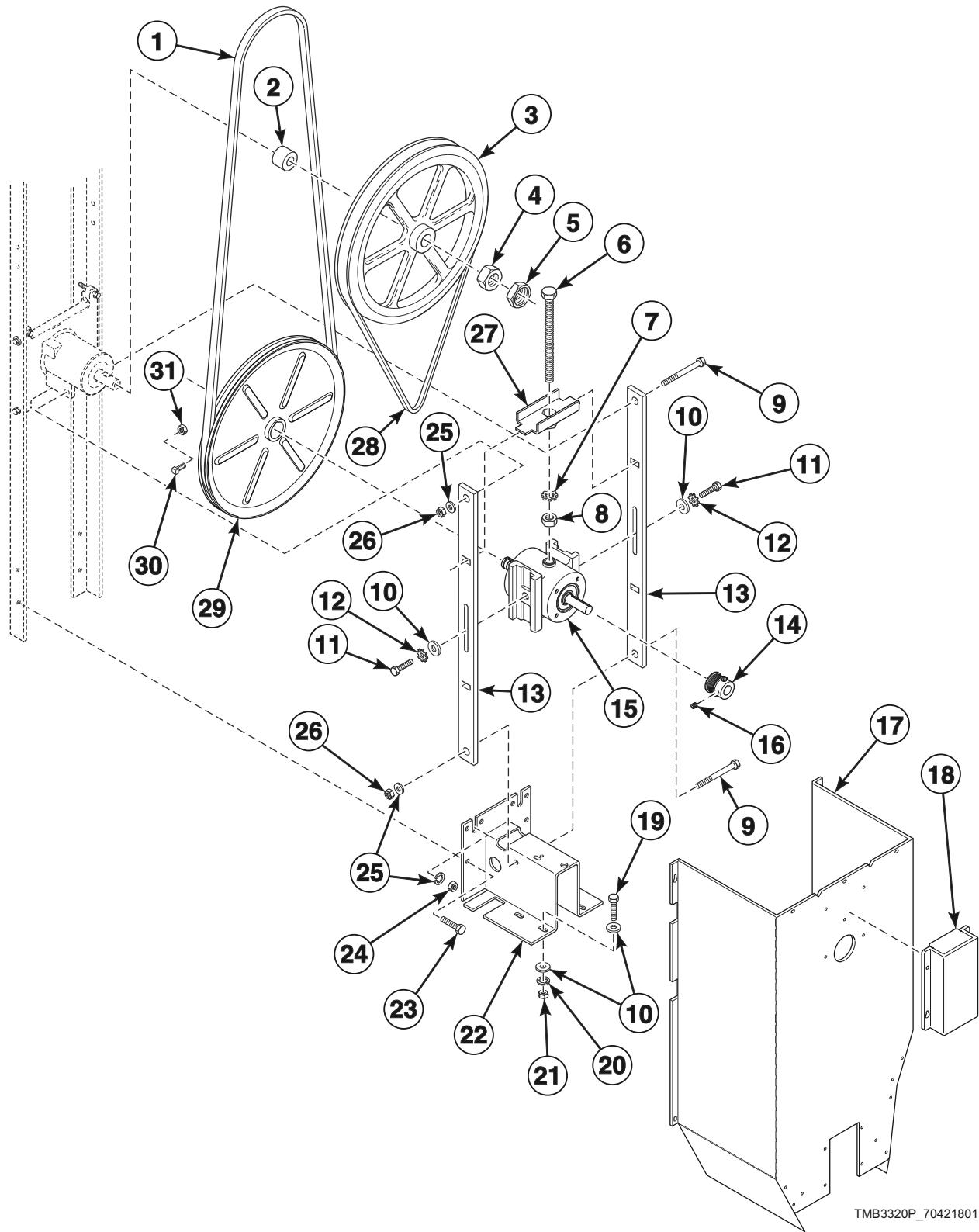
**Drive Components for Moisture Sensing Reversing Models**
