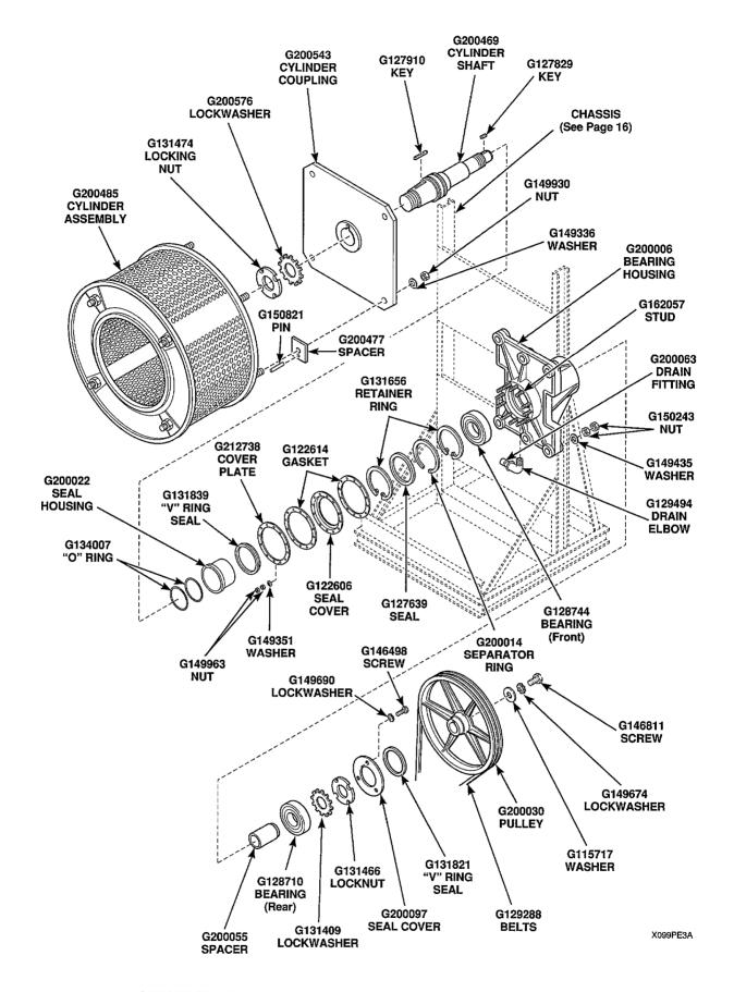
CYLINDER, SHAFT, BEARING HOUSING, PULLEY AND BELTS
